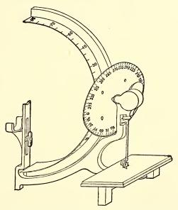
FIG. 9. Perimeter for Mapping the Retinal Zones.
