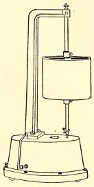
Fig. 30. Clockwork Kymograph.
