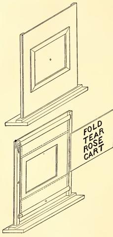
to 1G. 42. Demonstrational Tachistoscope. A black curtain, mounted on strong spring rollers, is stretched behind a square opening in a black wooden screen. The upper Fig. (front) shows the curtain and the white fixation-mark. The lower Fig. (back) has the card-carrier thrown back to show the square opening in the curtain itself.
