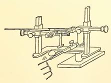
FIG. 31. Franck's Volumetric Sphygmograph (mechanical transmission by means of a system of levers).
