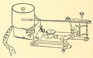
FIG. 37. Von Frey's Sphygmograph. The entire apparatus is bound upon the wrist, the button at the extreme right resting on the artery. The movements of the writing-lever are recorded on a very small, light drum, driven by a clockwork which is housed in the square box to the left. The clockwork also actuates a time-marker, shown in the Fig. at the lower edge of the drum.
