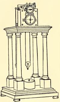
Fig. 62. Hipp's Chronoscope, an electrical clock whose unit is I σ: commonly employed in the reaction experiment.
