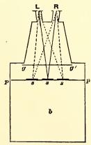
FIG. 53. Hering's Binocular Colour Mixer. L, R, the two eyes; b, dark box; gg', coloured glasses (red and blue); pp, supporting plate of clear glass; sss, squares of white paper.—Hermann's Hdbch. d. Physiol., iii., I, 1879, 593.
