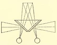
FIG. 49. Plan of Wheatstone's Stereoscope.
