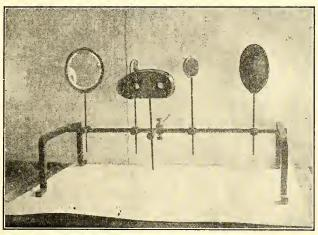
FIG, 51. Demonstrational Stereoscope, Telestereoscope and Pseudoscope.
