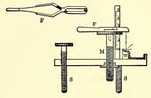
FIG. 26. Accounter for determining the Stimulus Limen of Noise. SS, setactives (two of the three are shown), supporting a wooden platform. M, mierometer screw at the centre of the platform, with scale beside it. FF, spring forceps, lying on the head of M, and carrying a small shot for dropping on the glass plate above W. The shot rebounds, and falls noiselessly into a padded trough.
