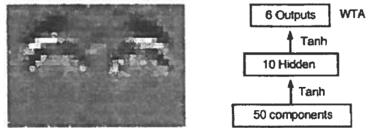
Figure 3: Left: Example difference image. Input values of -1 are mapped to black and 1 to white. Right: Architecture of the feed forward network.
